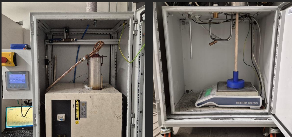
Figure 1: CO-TG test rig, developed by Forschungsgemeinschaft Feuerfest e. V.: the cylindrical reaction chamber with gas inlets on top of the tube furnace (left) and the weighing chamber with the sample holder placed on a precision scale (right).
