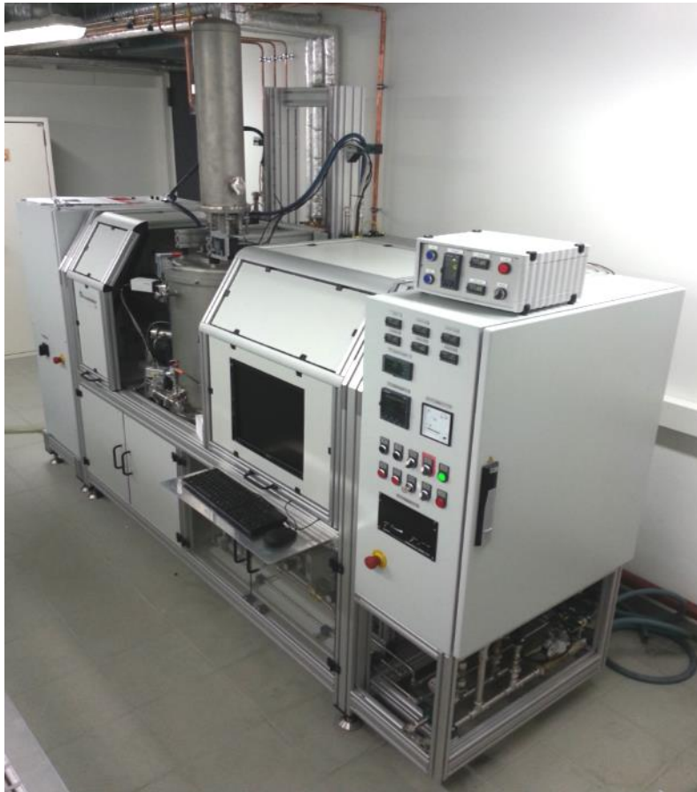
Fig. 6: Experimental testing device, showing the autoclave furnace equipped with a press and a system to control the atmosphere.
