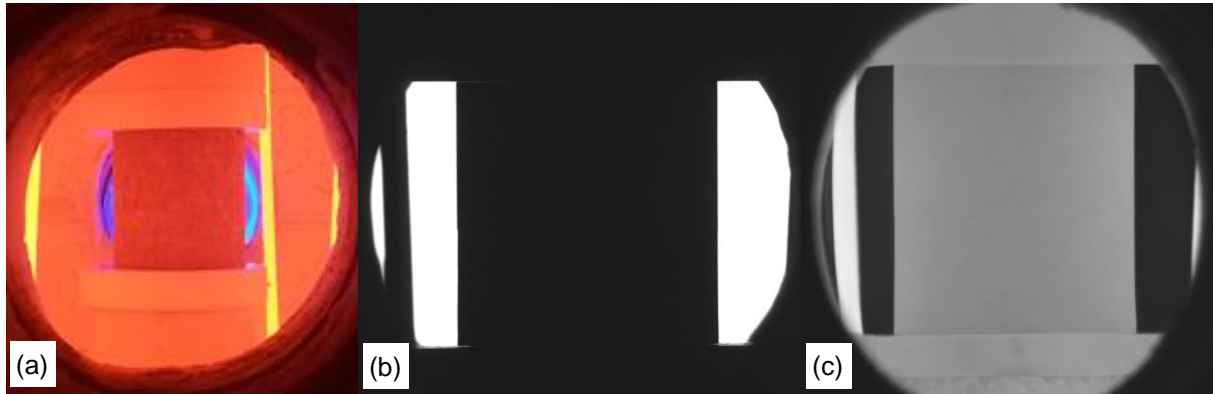
Fig. 7: Sample in the centre of the experimental furnace (a) at 700 °C. Images of the CMOS camera (optical dilatometer) (b) at room temperature (shadow of the sample), and (c) at 1500 °C (radiation of the sample).
