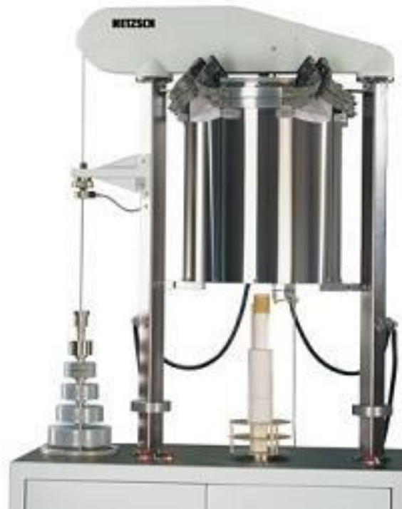
Fig. 3: Creep equipment where the applied load is the furnace itself and is regulated with a counterweight (source: Netzsch).
