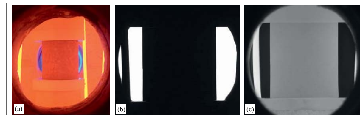
Fig. 1 36 mm × 36 mm refractory sample in the centre of the innovative testing equipment (a) at 700 °C. Images of the CMOS camera (optical dilatometer) (b) at room temperature (shadow of the sample), and (c) at 1500 °C (radiation of the sample)
